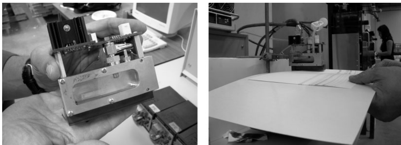
Figure 1 Spectra Nova print head (left) and passing a substrate under the running print head (right).
